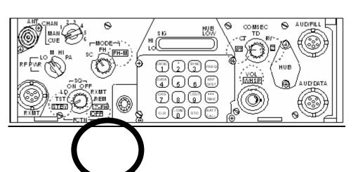
sc (single channel) places the RT in the single channel mode of operation. <u>COMSEC Switch</u> - sets the RT to the COMSEC mode. This switch has five (5) settings that allow the operator to use or manage COMSEC data (see figure 4).
