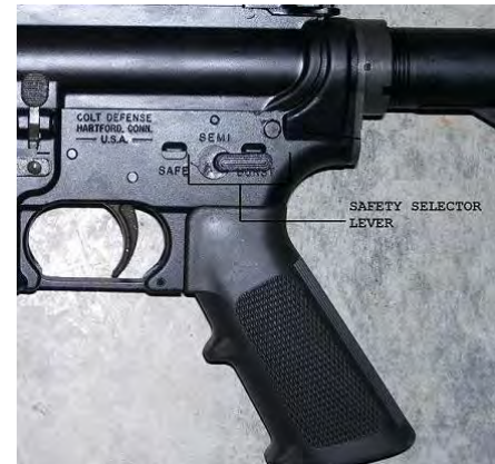
Figure 4. Selector Switch on Safe
