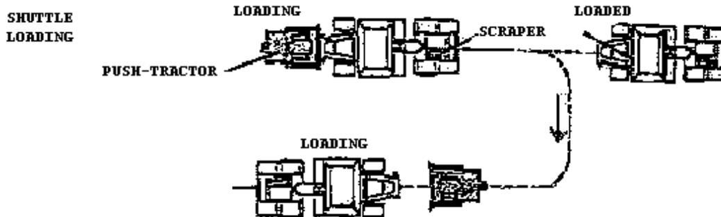
(a) The dozer pushes the scraper in one direction to the end of the dig pit.
